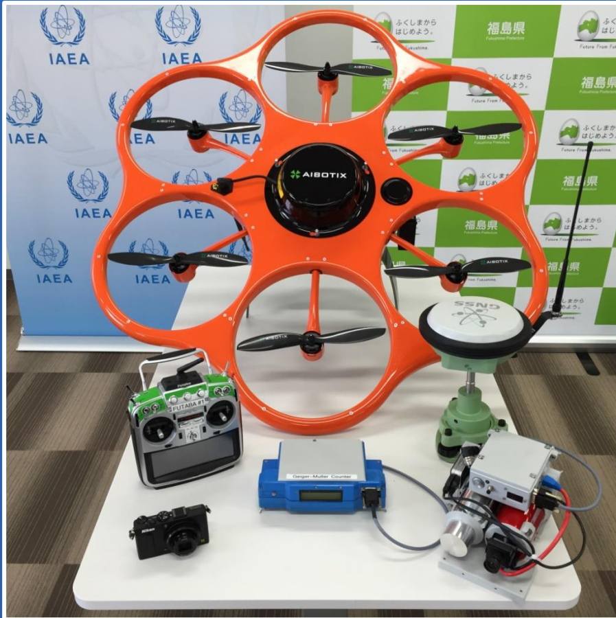
UAV (Aibotix) based system and its instrumentation components delivered to the Fukushima Prefecture.
