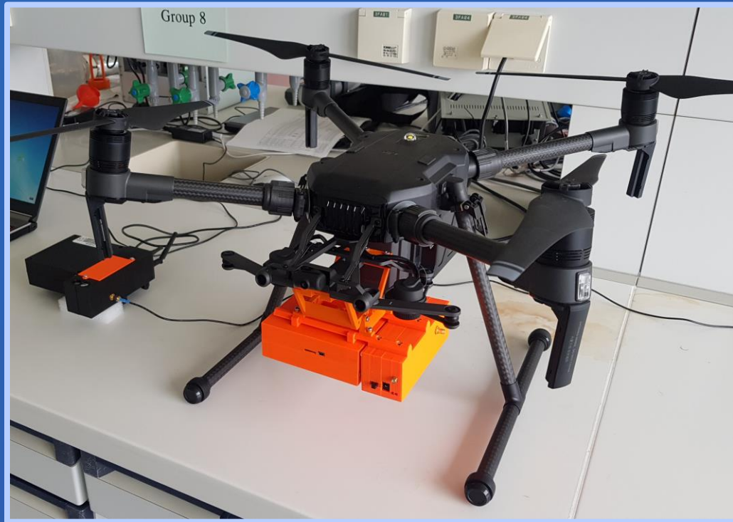
UAV DJI Matrice 210 V2 equipped by commercial GS module 1x1" SiPM NaI(Tl)
