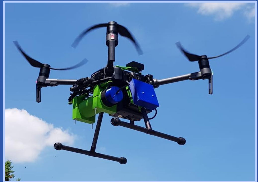
UAV DJI Matrice 210 V2 equipped by experimental GS module 2x2" NaI(Tl) & 1.5x1.5" SiPM CeBr3
