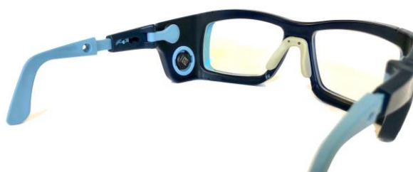
Figure 10.3: Eye lens doseimeters integrated into radiation protection glasses (Hoedlmoser et al., 2019b)
