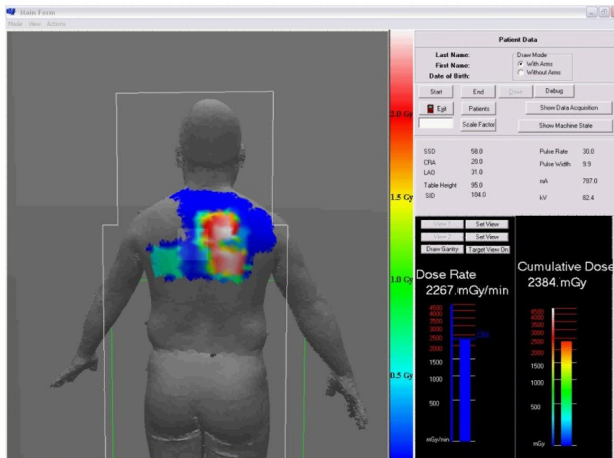
Figure 2.1. DTS display at end of a cardiac procedure showing the color-coded mapping of skin dose over the back of the patient (Bednarek et al., 2011)
