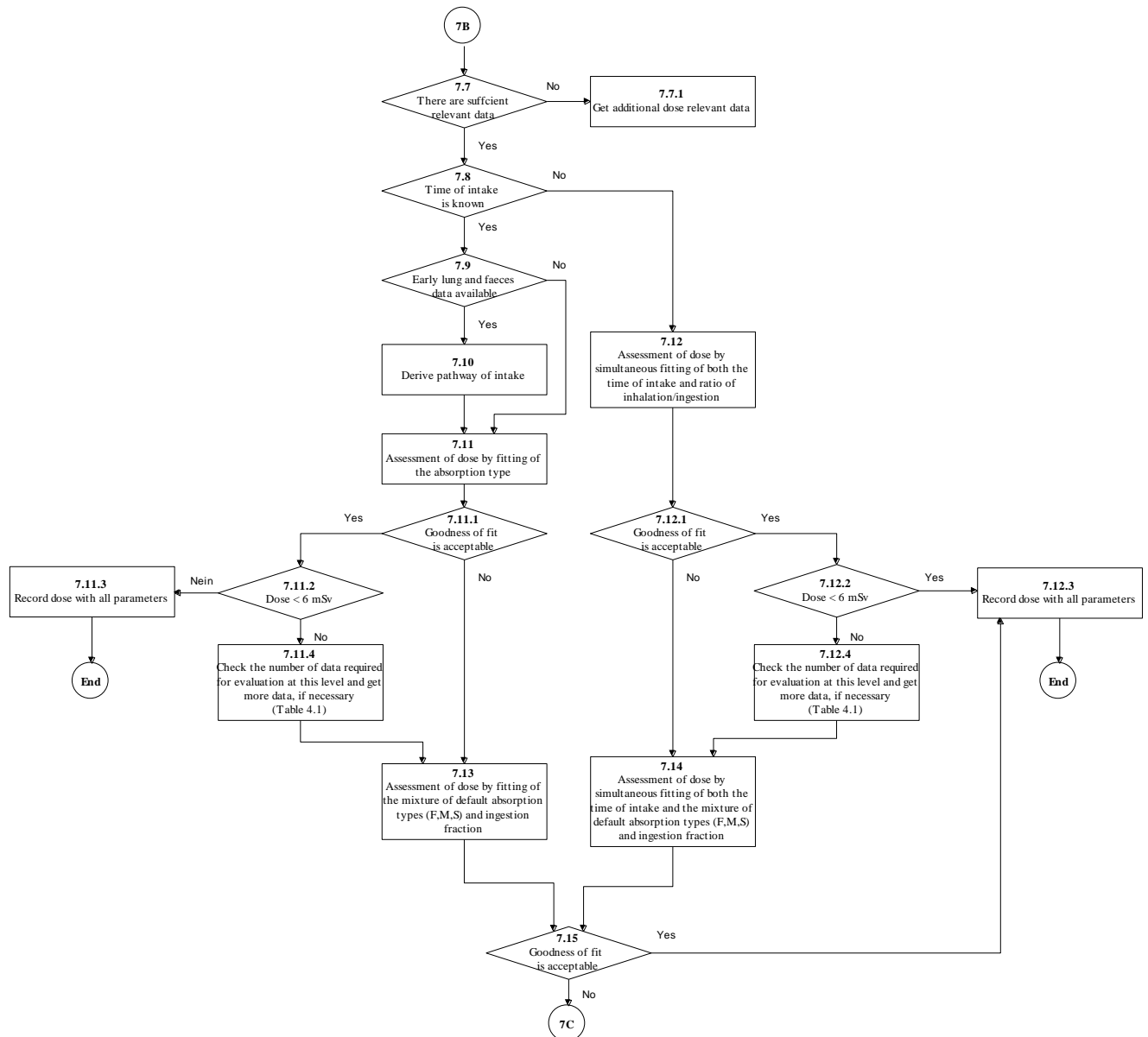
Figure 10.4: Stage 7B. Special procedure for mixed inhalation and ingestion cases above Level 1 – Part 2: Variation of the absorption Type and the ratio inhalation/ingestion, and also the time of intake, if not known.
