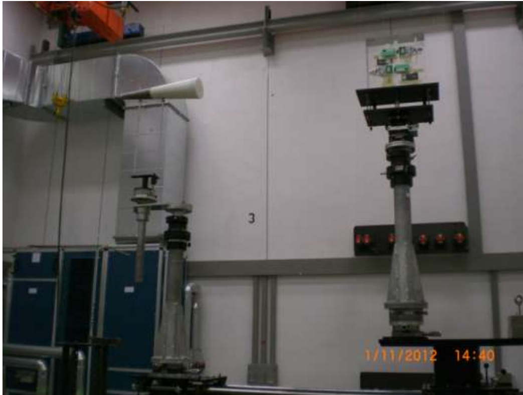
Figure 6: The neutron irradiation geometry for ^{252}\text{Cf} irradiations behind shadow cone
