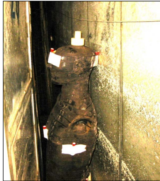
Tissue-equivalent anthropomorphic phantom fitted with dosimeters and positioned in the irradiation room
