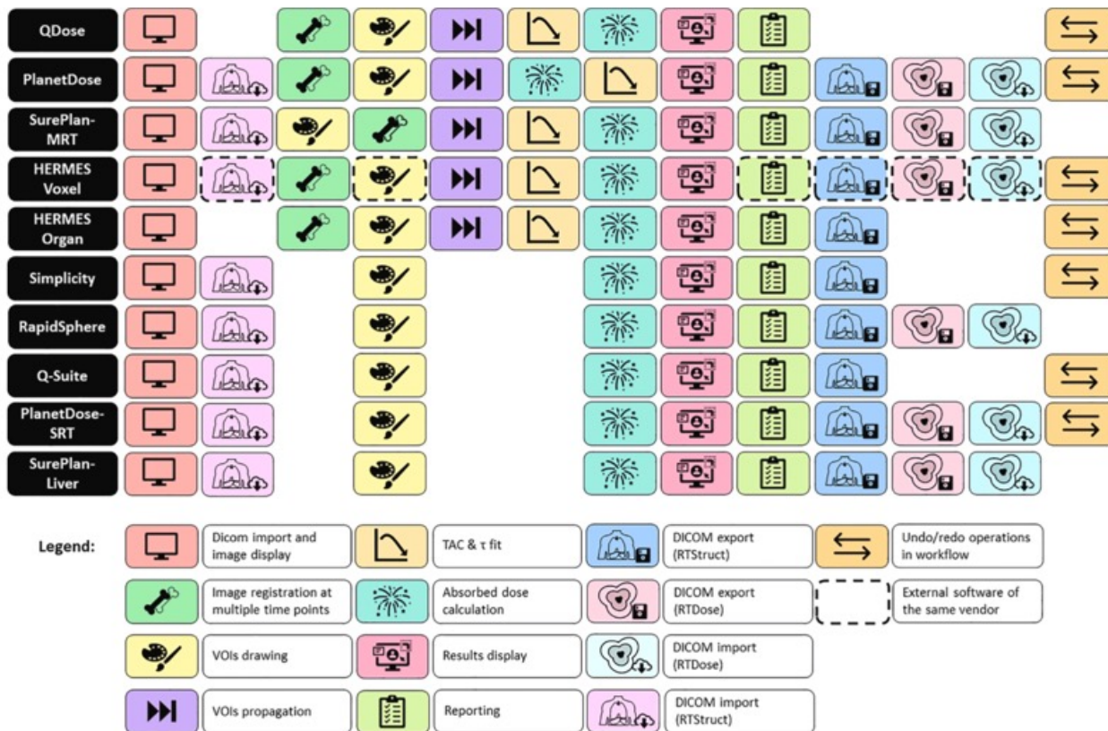
Fig. 1. Diagram of the proposed workflows in MRT and SRT TPSs. Workflow personalization is available for several TPSs.
