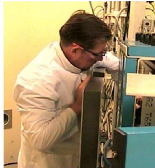
Replacement of cyclotron target © GE Healthcare, 2017
