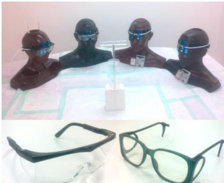
Figure 1. Set-up with four Alderson head phantoms (above) and protection glasses (below): laboratory glasses (left) and X-ray goggles (right).
