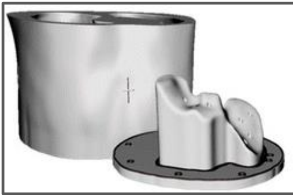
Figure 1: Division of the kidney into 4 separate parts to enable the fused deposition modeling 3D printing. A: CAD model. B: Printed parts.
