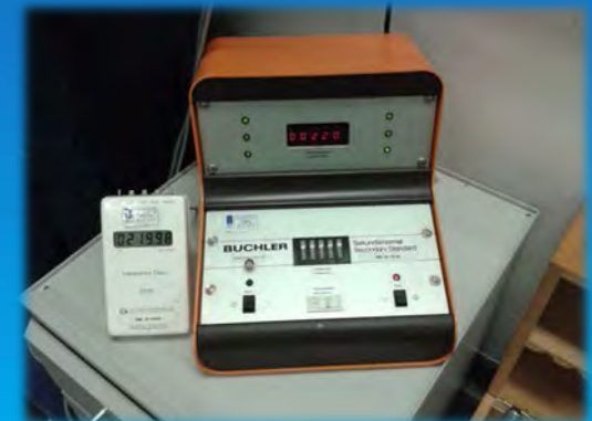
Sr-90/Y-90 source Nr. 23/50mCi fitted in the source stand. (No beam- flattening filter)
