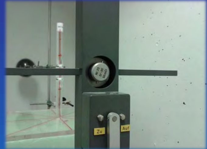
Sr-90/Y-90 source Nr. 23/50mCi fitted in the source stand. (No beam- flattening filter)
