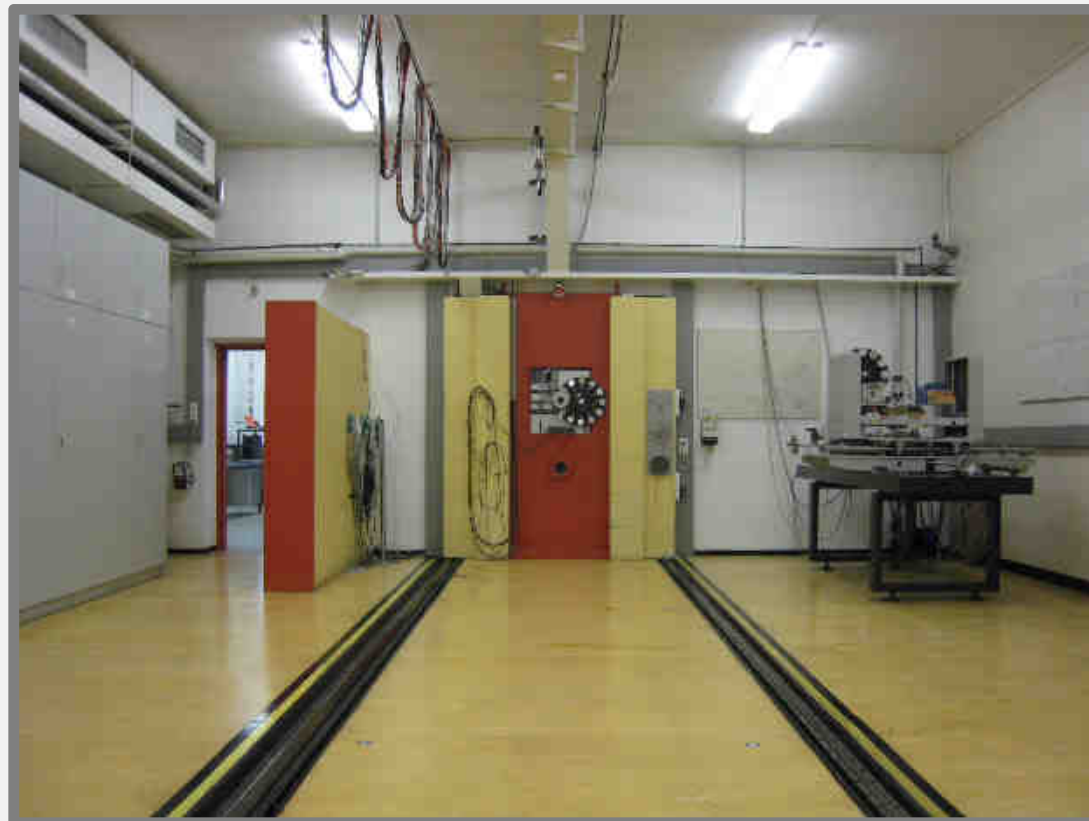
Measurement hall (320 kV X ray unit, ^{137}\text{Cs}/^{60}\text{Co} reference facility)
